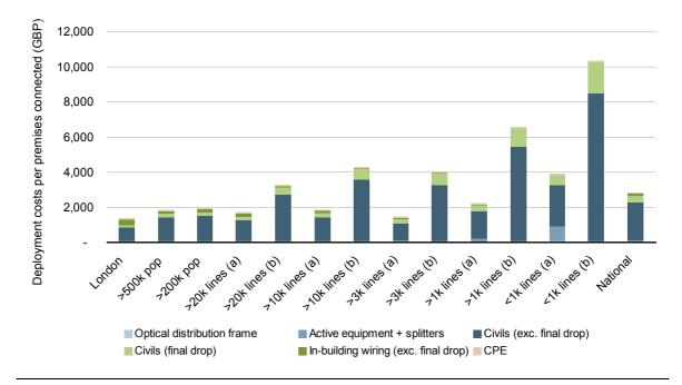
Figure 4.3: Breakdown of FTTH/GPON costs per premises connected [Source: Analysys Mason for BSG]
