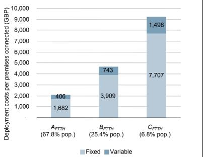
Figure 5.3: Fixed and variable costs per premises connected for FTTH/PTP split by geographical area [Source: Analysys Mason for BSG]
