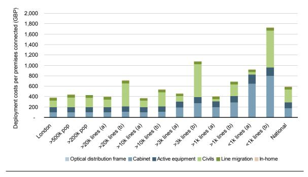
Figure 4.2: Breakdown of FTTC/VDSL costs per premises connected [Source: Analysys Mason for BSG]
