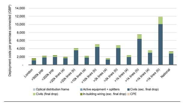
Figure 4.4: Breakdown of FTTH/PTP costs per premises connected [Source: Analysys Mason for BSG]
