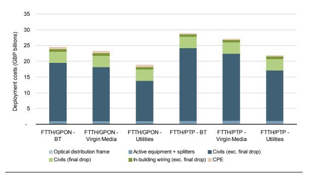
Figure 4.26: Deployment costs for a national network the different infrastructure scenarios for FTTH/GPON and FTTH/PTP [Source: Analysys Mason for BSG]
