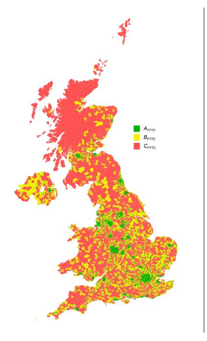
Figure 1.11: Map of the UK by area type for FTTC/VDSL [Source: Analysys Mason for BSG]
