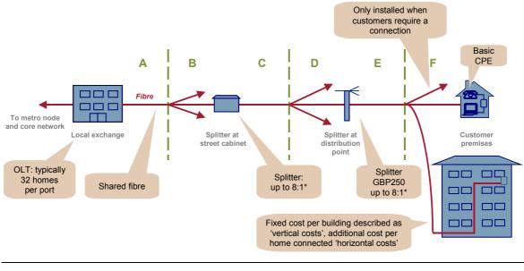
\*A single splitter can have a split of up to 8:1, but we would propose an overall split of 32:1 across both the cabinet and distribution point
