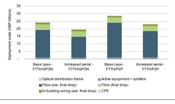
Figure 4.23: Impact of increased aerial deployment on a national basis for FTTH/GPON and FTTH/PTP [Source: Analysys Mason for BSG]
