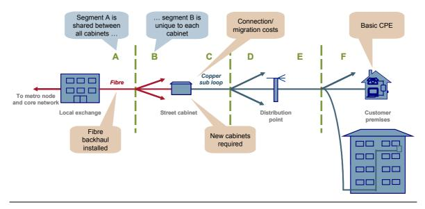
Figure 3.1: FTTC/VDSL network topology [Source: Analysys Mason for BSG]
