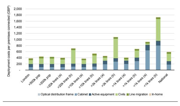
Figure 1.2: Breakdown of FTTC/VDSL costs per premises connected [Source: Analysys Mason for BSG]
