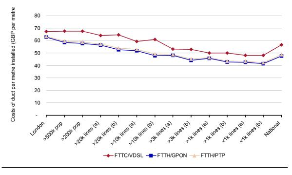
Figure A.8: Average costs of constructing new ducts [Source: Analysys Mason for BSG]
