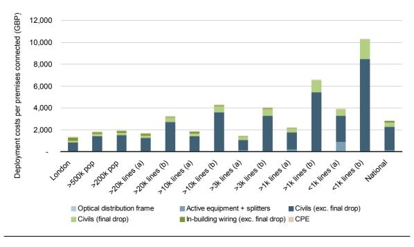
Figure 1.3: Breakdown of FTTH/GPON costs per premises connected [Source: Analysys Mason for BSG]
