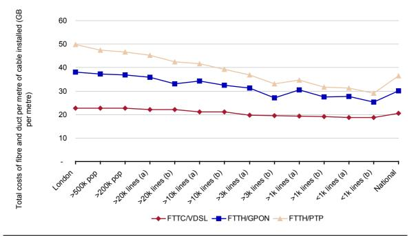
Figure A.9: Average cost per metre for fibre and ducts [Source: Analysys Mason for BSG]
