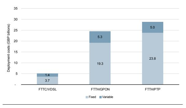
Figure 1.7: Costs for a national network split into fixed and variable costs [Source: Analysys Mason for BSG]
