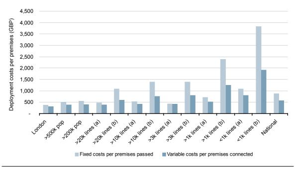
Figure 4.10: Fixed costs per premises passed and variable costs per premises connected for FTTH/PTP [Source: Analysys Mason for BSG]
