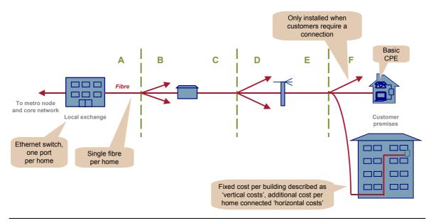
Figure 3.6: FTTH/PTP network topology [Source: Analysys Mason for BSG]
