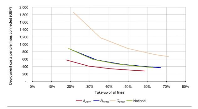
Figure 4.17: Impact of overall take-up on the costs per premises connected by area for FTTC/VDSL [Source: Analysys Mason for BSG]
