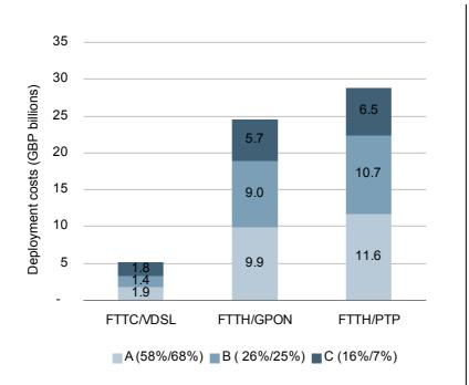
Figure 1.13: Deployment costs of each technology split by area (the corresponding population coverage for FTTC/FTTH is shown in parentheses) [Source: Analysys Mason for BSG]
