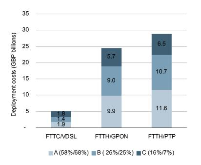
Figure 6.1: Deployment costs of each technology split by area (the corresponding population coverage for FTTC/FTTH is shown in parentheses) [Source: Analysys Mason for BSG]
