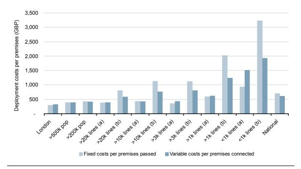
Figure 4.9: Fixed costs per premises passed and variable costs per premises connected for FTTH/GPON [Source: Analysys Mason for BSG]
