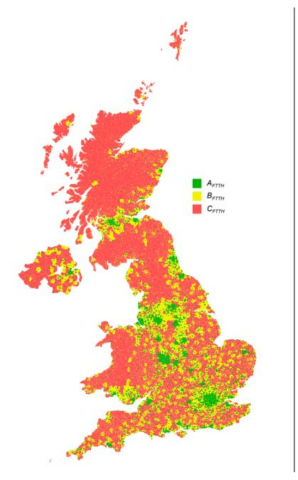
Figure 1.12: Map of the UK by area type for FTTH/GPON and FTTH/PTP [Source: Analysys Mason for BSG]
