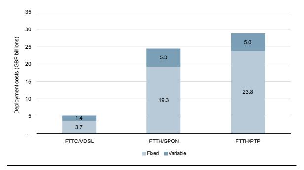
Figure 4.11: Costs for a nationwide network split into fixed and variable costs [Source: Analysys Mason for BSG]
