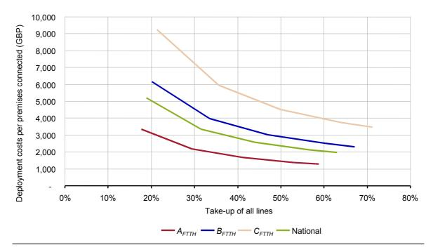
Figure 4.19: Impact of overall take-up on the costs per premises connected by area for FTTH/PTP [Source: Analysys Mason for BSG]
